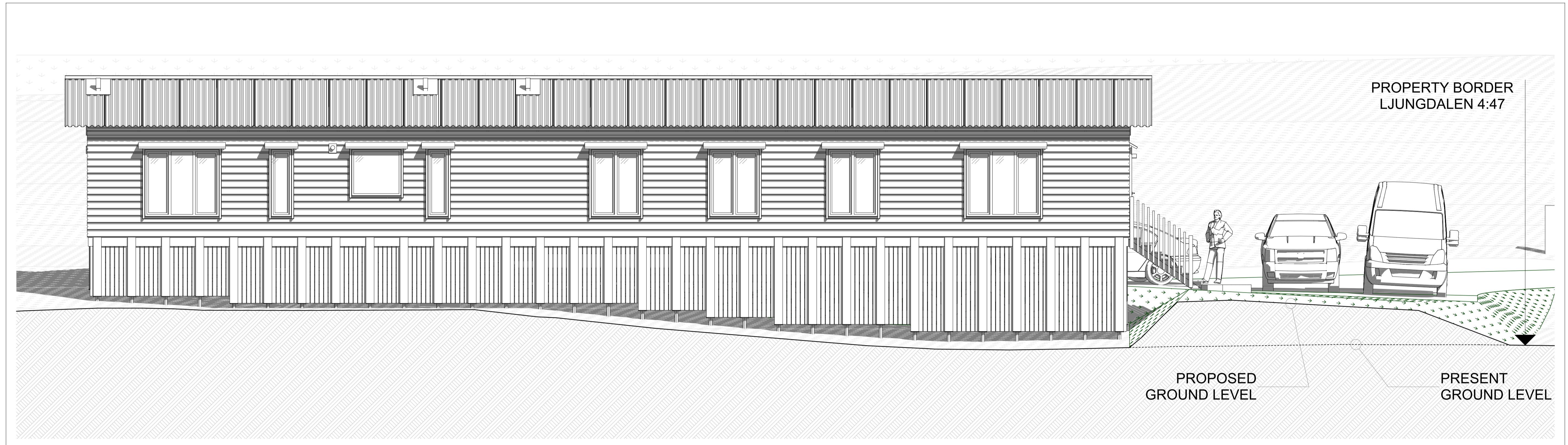
Facade F01 from east | approx. 2 meter outside logwall
